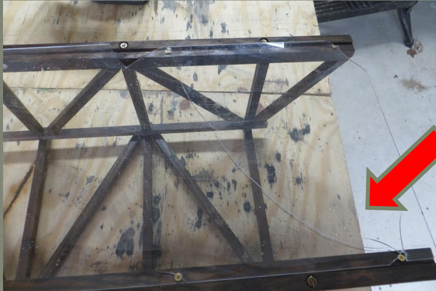
Large Triangular Corner Broke Free during transport
