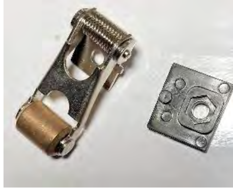
Pickup roller and plastic insulator
